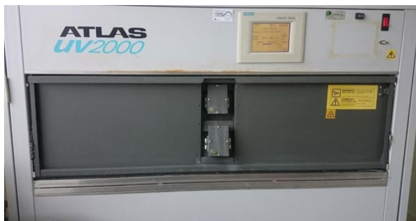
Figure 5. Atlas UV2000 Aging Device.
