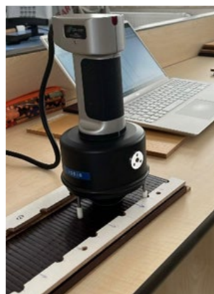
Figure 3. MINOLTA CR-231 color measurement device.
